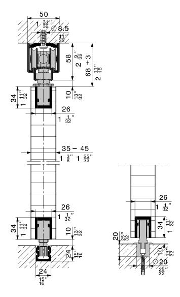
Flush partition walls with flexible folding.
