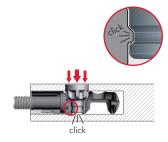
Press strongly with PZ2 cross screwdriver to slot the pinion screw in.
