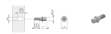
Note: Special threaded pin to avoid hole damging for shelf repositioning.
