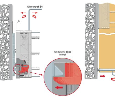
The Self-Inserting anti-turnover device is carried out after 3mm of in-depth adjustment
