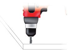
**3** - Screw the assembly fitting into the face bored panel using a cross screwdriver.
