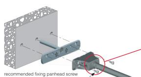
VERY IMPORTANT Triade Maxi has to be installed with the arrow facing upwards.
